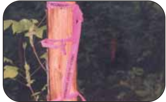
The two photos above are examples of Flagging ribbon—colored plastic "ribbon" in several colors and patterns.
