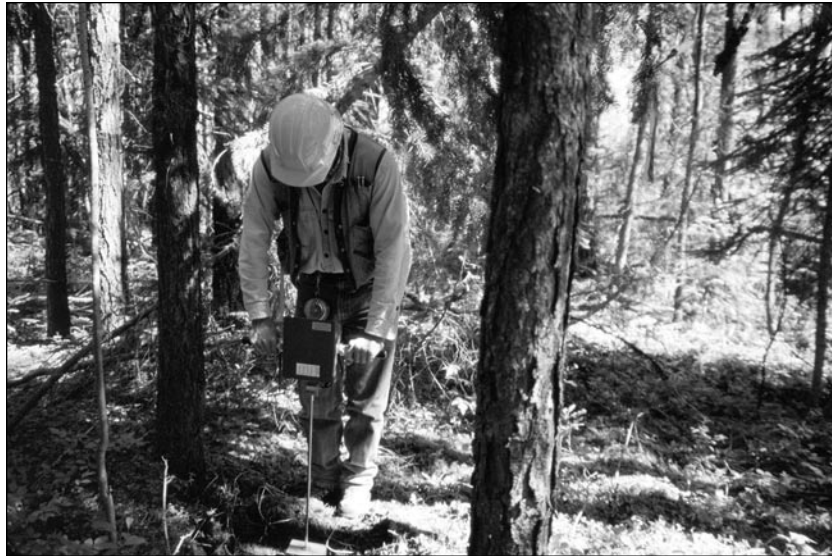
Figure 4—Soil resistance was measured with a recording penetrometer at each station.
